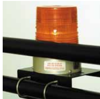
BS2 Light Mount Plate 6" x 9" steel plate with stainless steel "U"-bolts attaches to cross bars or side rails for beacon or strobe lights.
