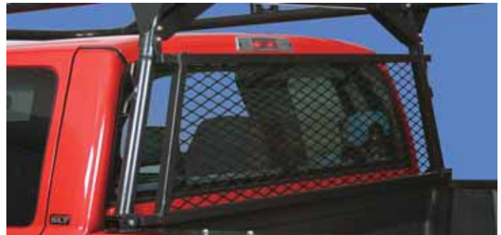
WG21 Window Guard/ Black or WG21W Window Guard/White Use with standard Load Runner for all Chevy/GMC/Ford Regular Duty pickups.
