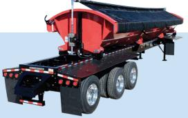
The proven best solution for side dump trailers. The patented tube and roller design works in unison with the industry's most reliable spring and motor technology to cover and uncover side dump loads quickly and consistently. Featuring the strongest roll tube on the market, the SideKick 2 side-to-side tarp system outperforms the competition.
