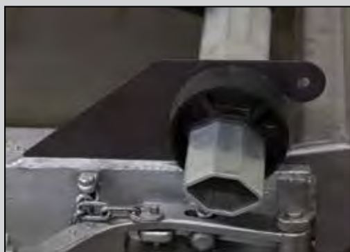
3029712 Carbon steel tension bow catch plate (optional 3029712SS stainless steel catch plate upgrade available)
