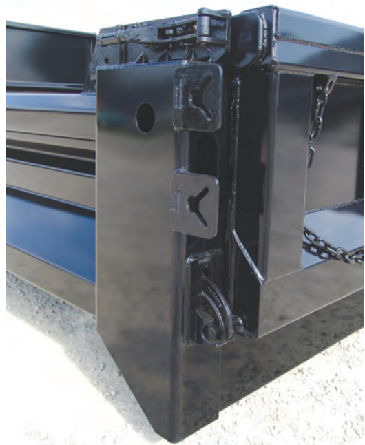
Pictured is a close view of the upper quick release hardware and banjo eyes of the standard PLD body. This hardware makes it easy to quickly remove and reinstall the tailgate as needed.
