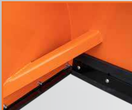
Rubber Edge 3/8" x 4" rubber edge mounting bracket, 1-1/2" x 10" premium rubber edge, 5/8-11, grade 5 carriage bolts
