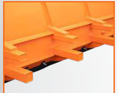
Reinforced Support 4" x 4" 3/16" lower posts and 3" x 4" x 3/16" upper posts with 72" wide x 4.5" tall post spacing
