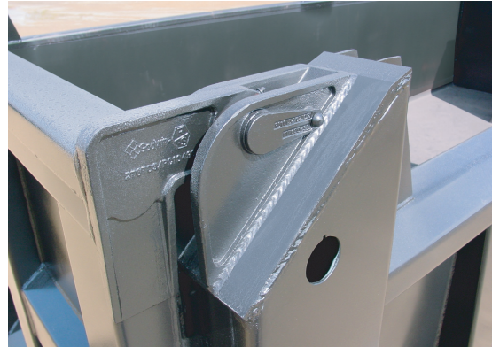
Pictured is a close view of the upper tarp friendly hardware of the standard 500U-T body. This hardware makes it easy to quickly remove and reinstall the tailgate as needed.
