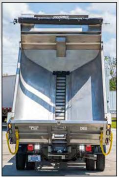
Cross member-free design makes the unit easy to clean with a low center of gravity that reduces strain
