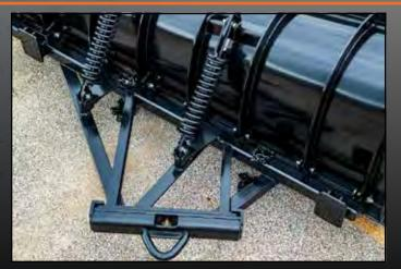
Full Length Push Frame with 4" Heavy Duty Structural Channel Push Beams, and 3-1/2 x ½ Outer Brace Angles
