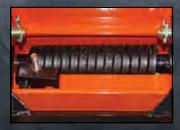
Trip edge design with 5 adjustable torsion springs
