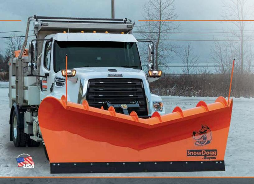
4-position attack angle adjustable trip from 0° to 20°
