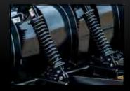
Full moldboard trip with two adjustable compression springs
