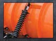
Full moldboard trip with two adjustable compression springs
