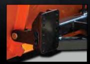
Standard mounting brackets for running gear
