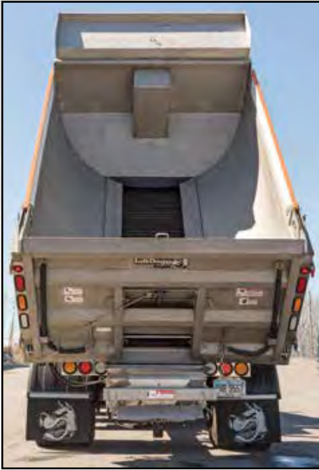
Unique, roll-formed sides and cross member-less design
