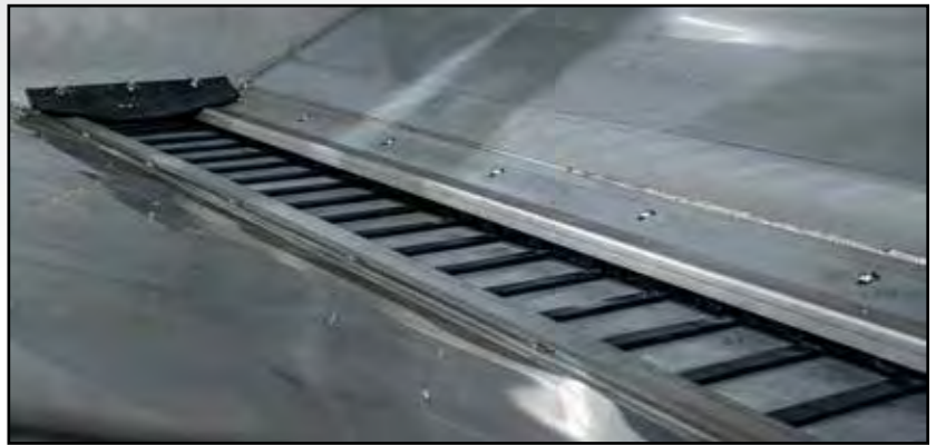
A high speed conveyor chain feed, 14-1/2" wide conveyor with 1/4" bars
