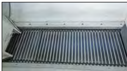
30.25" wide conveyor with 1/2" bars
