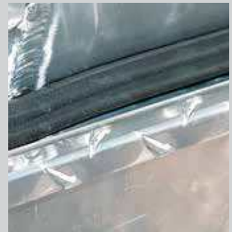
Full weather stripping keeps dust and moisture out
