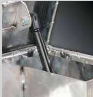
The cover support housing protects the gas shocks
