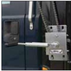
Tarp crank with friction brake
